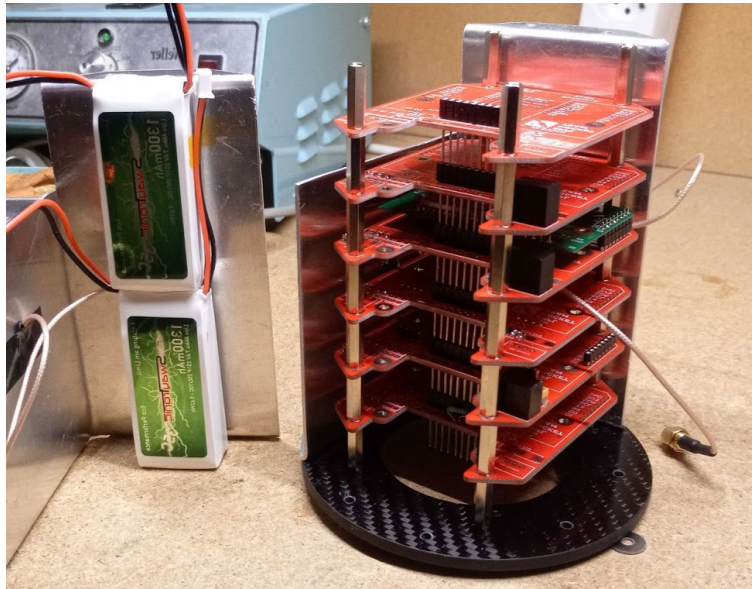
Figure 1: Avionic module with integrated IMU and barometer
